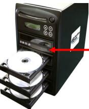
**Step 3**: Eject reader tray (top drive) and insert source disc. Close reader tray.
