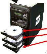
**Step 4**: Eject Recorder tray(s) and insert the blank disc(s). Close Recorder tray(s). Duplication will start automatically in 5 seconds.
