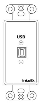
The Intelix USB-WP-series extenders transmit low speed USB 1.0 and 2.0 signals up to 330 feet, and full speed USB 1.0 and 2.0 signals up to 100 feet over twisted pair cabling. Decora inserts allow installation in any setting, facilitating a clean, low profile installation.
