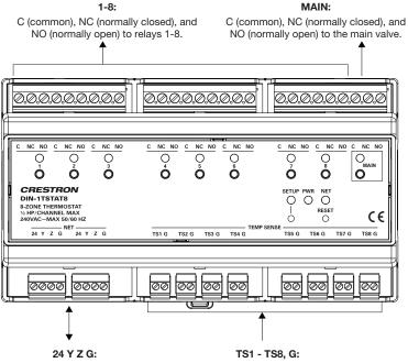
Cresnet control from a control system and to daisy-chained Cresnet device. TS1 - TS8, G: Temperature sensor input from remote temperature sensors
