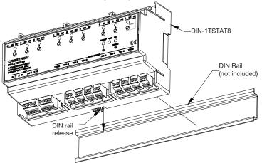
To remove the DIN-1TSTAT8 from the DIN rail, use a small, flat object (such as a flat-head screwdriver) to pull the DIN rail release tab down, and then tilt the bottom of the DIN-1TSTAT8 away from the DIN rail.
